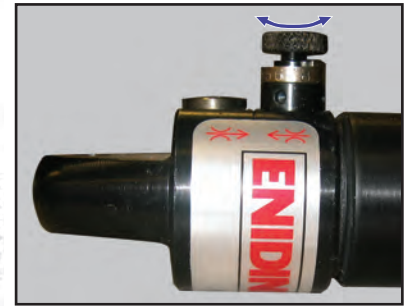
Position 0 provides minimum damping force. Position 8 provides maximum damping force. 180° adjustment with setscrew locking.
